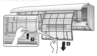
**3** Remove the titanium apatite deodorising filter and silver particle filter from the tabs.
